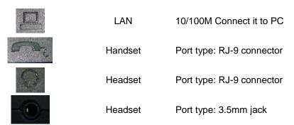
VPS-2000P provide two Ethernet ports and a power adaptor. Also has two headset interfaces with RJ-9 port and 3.5mm jack. Please refer to safety notes of this manual carefully before power adaptor is connected.
