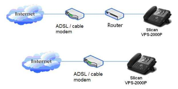
Shared network connection—Use this method if you have a single Ethernet port in your workspace with your desktop computer already connected to it. First, disconnect the Ethernet cable from the computer and attach it to the WAN port on the back of your phone. Next, use the Ethernet cable in the package to connect LAN port on the back of your phone to your desktop computer. Your IP Phone now shares a network connection with your computer. The following figure is for your reference.
